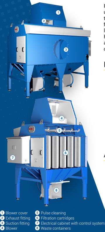
For most applications our filtration units enable air to be returned back to the production floor. Operators of the filter units must pay attention to local legislation relating to dangerous materials. For example, regulations regarding minimum allowable levels of fresh air supply and other country-specific regulations.
